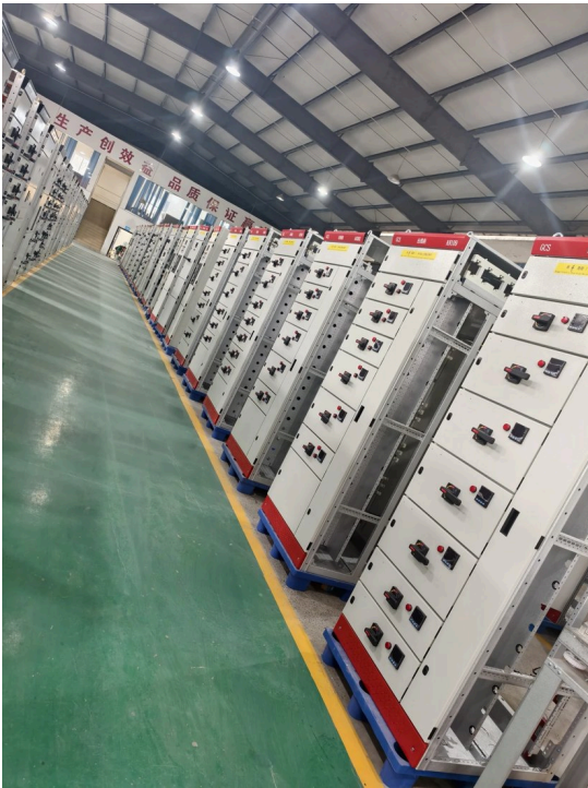
A modular low-voltage switchgear family for receiving and distributing power across industrial, commercial and municipal electrical systems.
